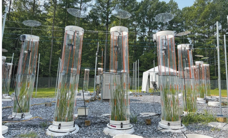
Open-top chambers, where scientists are growing wetland plants exposed to extreme events and measuring greenhouse gases.
